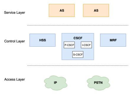
Figure 2.1: IMS High-level Architecture
