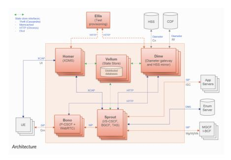
Figure 3.1: ClearWater Architecture, adapted from [Neta]
